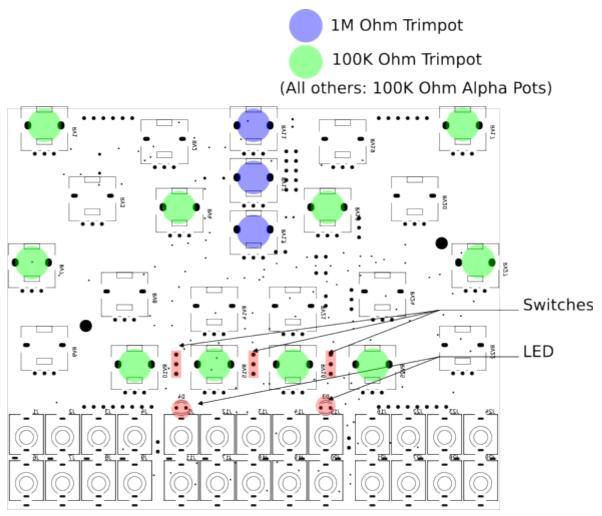
**Notes : LED insertion .** The smallest PIN into the square hole
