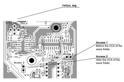
As for the MS processing, you have cut the circuit between the two holes, and solder a pinheaders or a wire.
