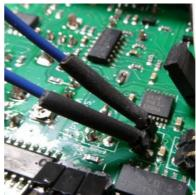
The MULTIPLE side. Note the cable soldered between the 2 jacks (« Norm » pin)
