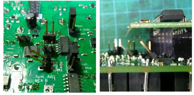
A good tip, for the pinheaders under the voice PCB : Soldering the PINs askew, because there is not a lot of space between the two PCB. (*Yes, I know, sorry for this bad design...*)
