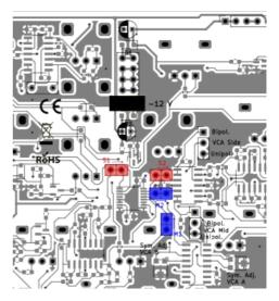
In my humble opinion, it's not necessary to use both M1/S1 and M2/S2. Just one is useful. - M1/S1 is **before** the selection MS or LR. This connexion is useful to add a treatment to the mid and side signal, without touching to the LR signal.
