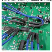
I recommend using heat shrink tubing to avoid short circuits
