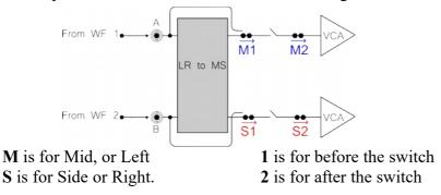
Both are very useful as insert point. To add treatments in the Mid/Side domain (Eq?). And also to bypass the LR to MS part of the processor. For example, you can connect the Voice 1 to the Mid, and the Voice 2 to the Side.
