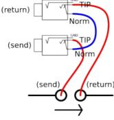
If you want to build an insert, use this condiguration : In this case, you will need two jacks. And if you do it for both circuit (M and S), you will need four jacks, of course. Note the cable between the two « Norm » pin.
