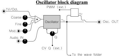
The oscillator is designed to generate a sine signal. For this purpose, the circuit is almost similar to a filter. Electroncialy speaking, it's a controlled feedback loop. It means we can use it as a VCF. Two controles are added :
