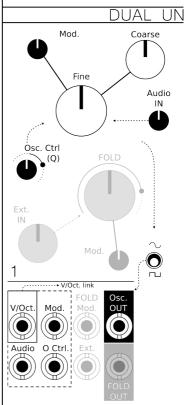
The waveform is selected by the switch under the Wave folder
