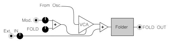
The effect of the wave folder depend on the amplitude of the input signal.
