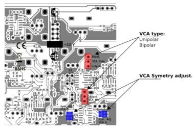
As already explained, each VCA can be configured as unipolar (classical VCA) or bipolar (default configuration), with the jumper :
